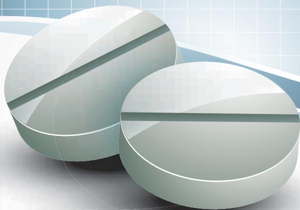
**TABLET SCORING** has long been used by oral solid dosage manufacturers—originally as a means to prevent tablet stress fractures, but recently as more of a cosmetic feature [1]. Bisects, of course, present manufacturing challenges. They “may be affected by the tablet cup depth, band thickness and the intended tablet hardness. As the tablet size increases or changes, so do the size and type of bisects that may be placed” [2,3].
