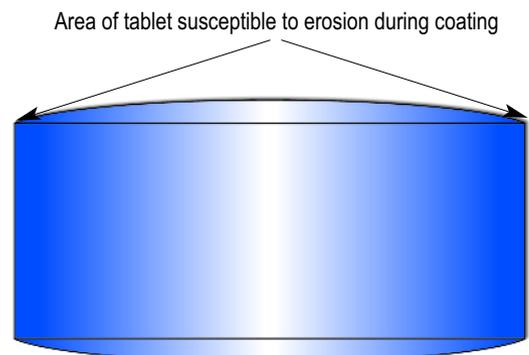
plement). For this tablet, let's say the deepest part of the cup may be 0.060 inch. Following the published standard, the acceptable range would be 0.057 to 0.063 inch. But because the cup is deeper than the one used to make the small tablet, the percentage range of deviation is substantially less: 10 percent. That is a considerable difference, the importance of which is magnified by the fact that this small-diameter tablet is a Schedule II pharmaceutical product.
