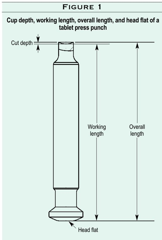
Understanding the working length leads to consistent overall tablet hardness, weight, and thickness, so it should be considered the most important dimension in a tool inspection program. If the working length varies, then tablet hardness, weight, and thickness will also vary.
