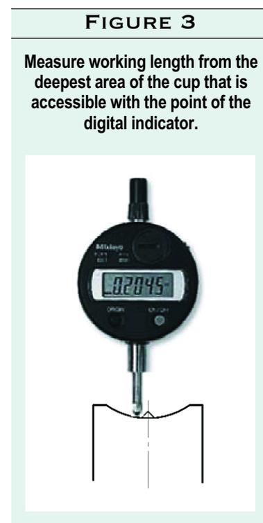
Whatever equipment you use, measuring the working length of punches that have embossing or a bisect at the lowest area of the punch cup is more complicated. In those cases, it's important to measure from the deepest area of the cup that is accessible with the point of the indicator (Figure 3). Once you identify the lowest area of the cup, be sure you consistently measure from there as you check the entire set. Otherwise, you may have to "hunt and peck" for the lowest area of the cup.
