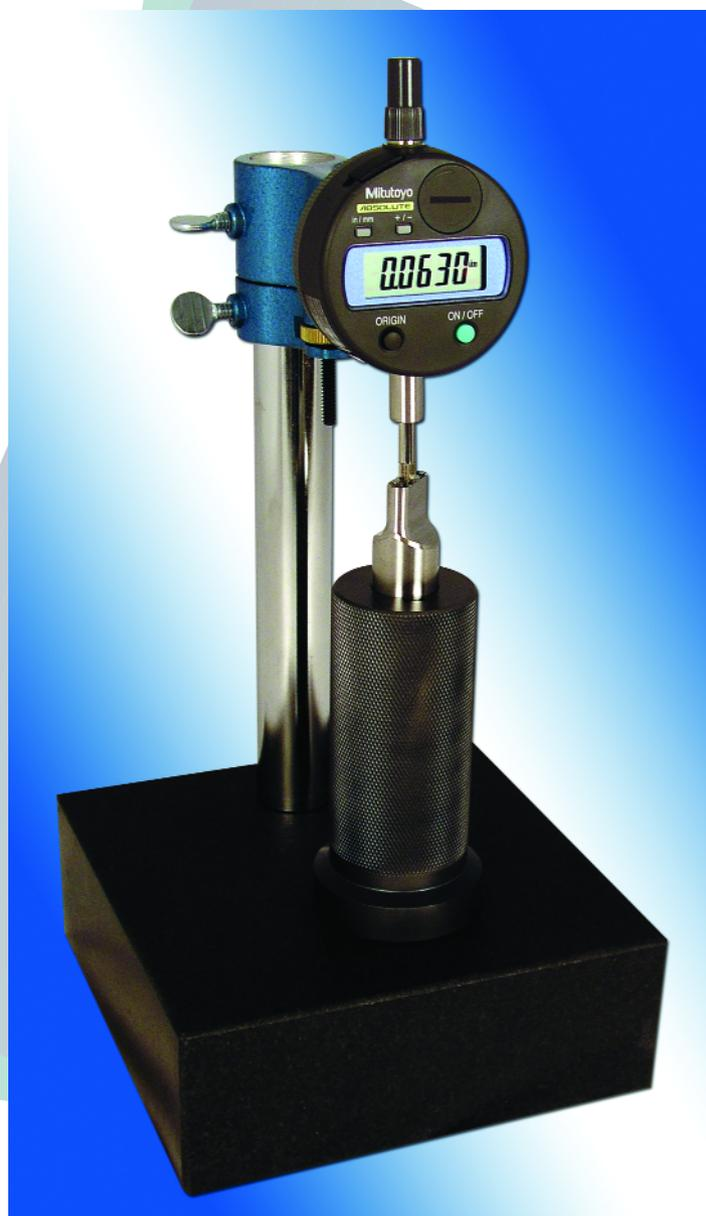
*Manufacturing tablets to a uniform hardness, weight, and thickness requires tablet press punches of consistent length. This article describes how to understand punch length, how to measure it correctly, and how wear affects length and tablet consistency. The article also addresses the importance of specifying cup-depth tolerances.*
