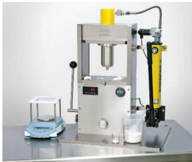
A single-station tablet press for conducting compression studies [1]
