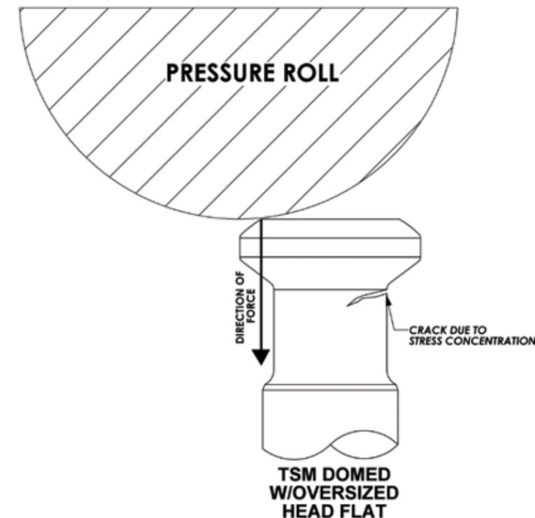
FIG. 2: A head with a stress crack
