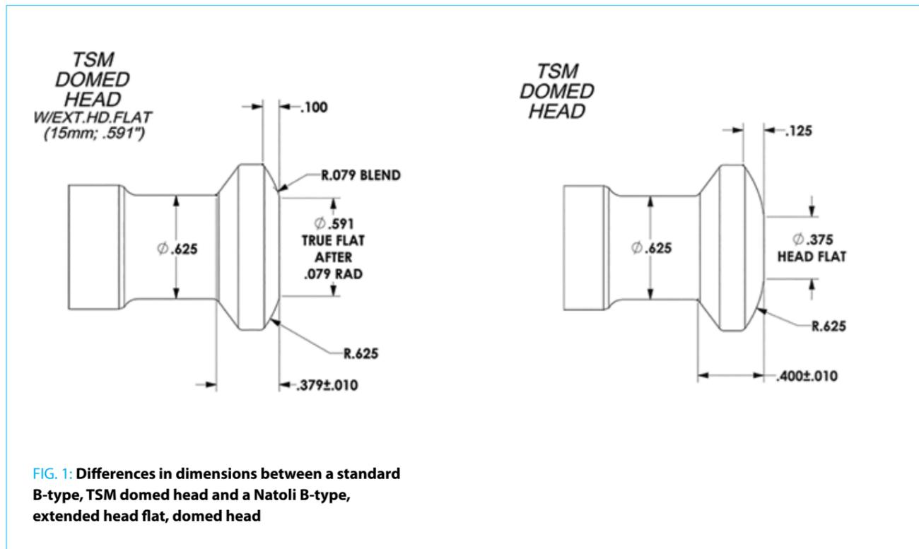
FIG. 1: Differences in dimensions between a standard B-type, TSM domed head and a Natoli B-type, extended head flat, domed head
