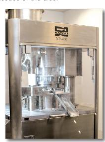
er-speed motor, redesigning the feeder paddles, and lowering the paddles closer to the dies. These changes increased production speeds and improved the tablet consistency issues.
