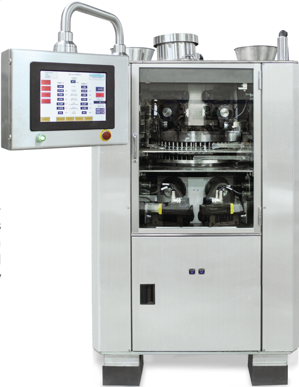
Reconditioned Kikusui press with enhanced control system.
