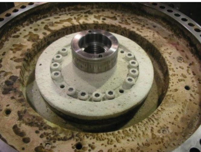
Figure 3. Contaminated spindle bearing.
