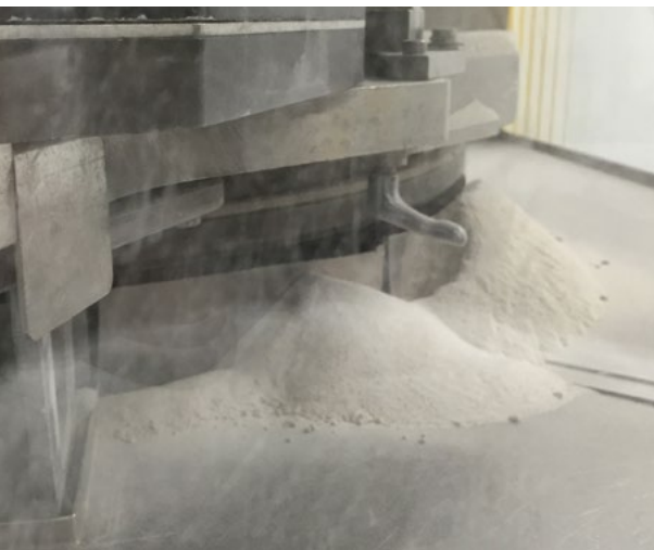
Figure 1. Excess formulation on die table.
