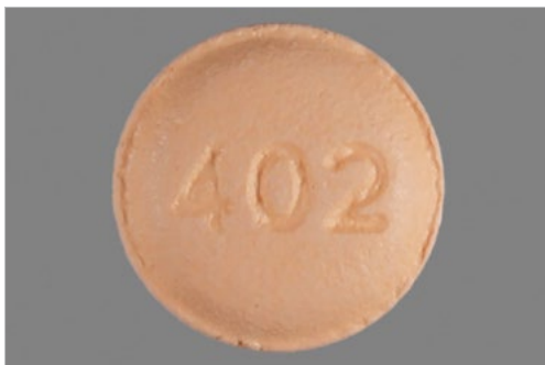
Figure 2. Excessive flashing on tablet
