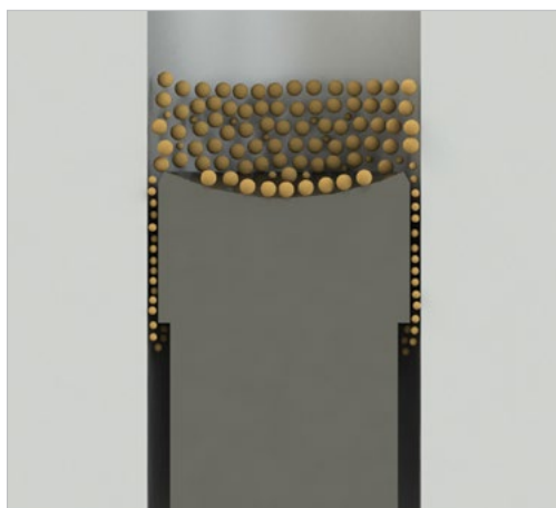
Figure 3. Tip wear on outer die edge and small particle sifting inside die bore.
