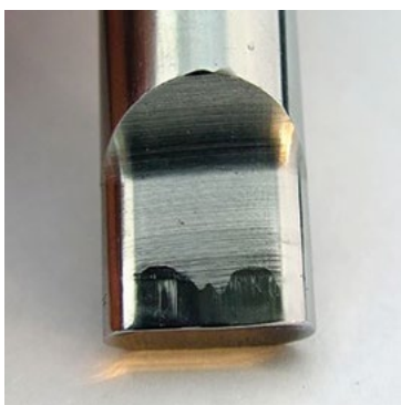
Figure 5. Resulting damage to punch tips
