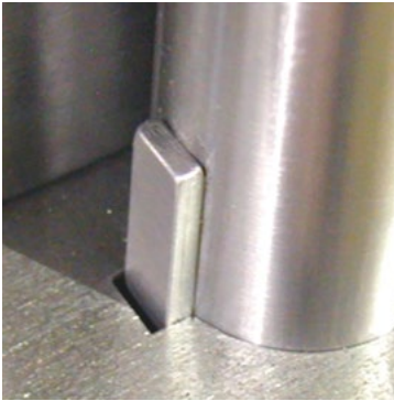
Figure 9.1. Punch key not pre-loaded.
