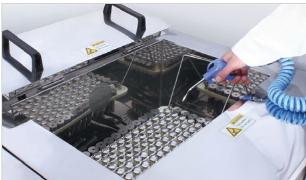
Proper drying prevents rust, which can severely damage your tooling.
