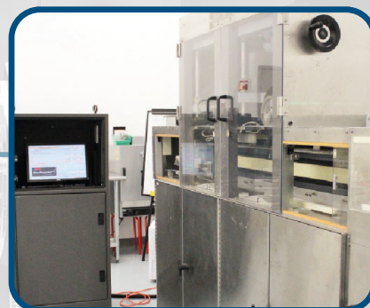
Presster Measure punch displacement, calculate tablet volume and display Heckel or stress vs. strain under high speed conditions
