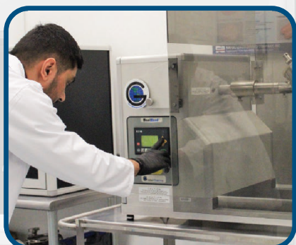
GlobePharma V-Shell Blender Setting parameters for powder blending
