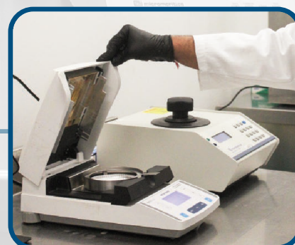
Mettler Toledo Moisture Balance & Micromeritics Helium Pycnometer Sample moisture balance for loss on drying testing
