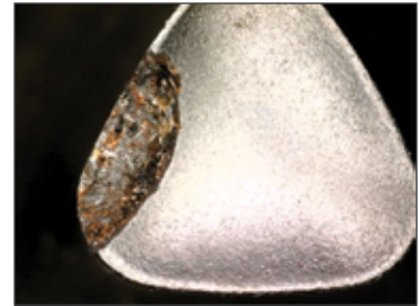
Punch Tip Damage Photo Taken with IN 7951
