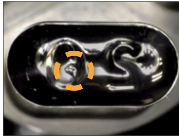
Punch Tip Damage Photo Taken with IN 7951
