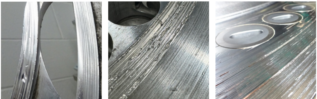
Examples of die table and feeder damage from improper leveling:
