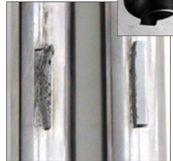
Damage to key from excessive wear
