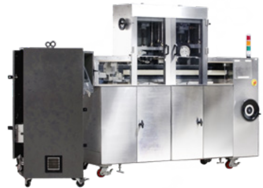
The Presster can test a single tablet at production speed from a library of press models.
