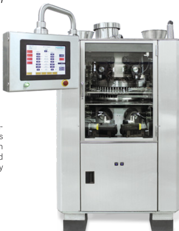
Reconditioned Kikusui press with enhanced control system.
